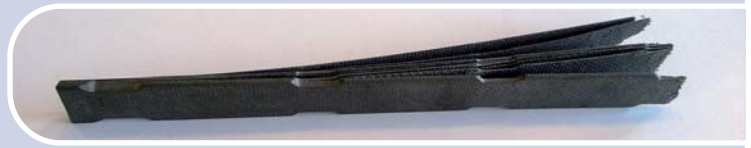
Picture 5: above: In the picture you can see a laminated magnetic slot wedge with poor adhesion between the layers, so that even small forces lead to delamination.
