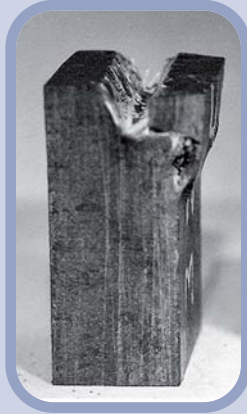
Picture 5: above: In the picture you can see a laminated magnetic slot wedge with poor adhesion between the layers, so that even small forces lead to delamination.
